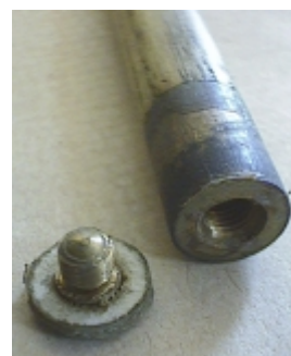
An early example of a screw-in tip which began to become popular in the late 1880s
